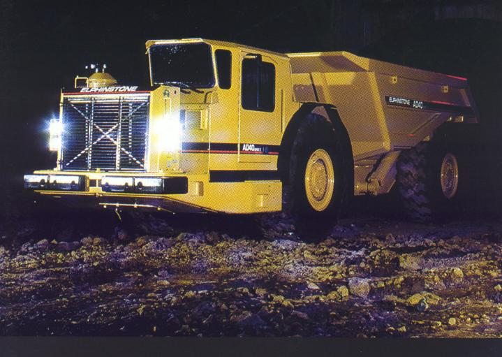
CAT® 3408E HEUI Engine Gross Power 365 kW (490HP) Rated Load 38,800kg (85,554lbs) Operating Weight 82,100kg (181,030lbs)
