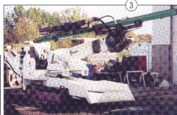
3. TDM with drill boom and both electric and diesel motors, Dragon Mount Mine, China 4. Discharge of spoils from rear conveyor
