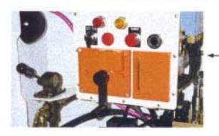
Trojan MT operator controls are ergonomically located allowing easy reach to controls, braking, and information.
