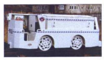
Warren's new gear drive enables extremely high power densities with very high safety factors enabling the production of compact locomotives. This narrow drive design enables an integrated suspension system for those tight tunnelling applications behind TBM's in gantries and backup units. In mining where chutes are low and dumps are in narrow areas, this design allows a powerful yet compact locomotive to improve productivity safety.
