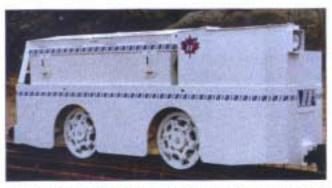
A DC motor for battery and trolley locomotives powers each worm gear drive. When diesel operation is required, variable displacement hydraulic pumps supply fixed displacement hydraulic motors. DC drives are managed with proven dual motor Mosfet controls with many safety and preventative maintenance features. Diesel drives feature simplified PLC controls for safe acceleration and deceleration.
