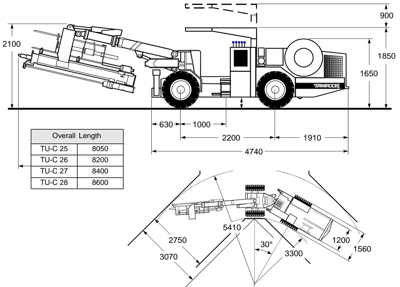
**Highly compact rock bolter, four wheel drive hydraulic jumbo, for installation of bolts from 5 to 8 ft in drift of height up to 4.8 m.**
